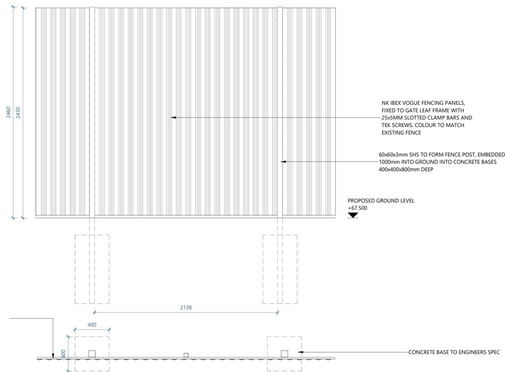
NK IBEX VOGUE FENCING PANELS, FIXED TO GATE LEAF FRAME WITH 25x5MM SLOTTED CLAMP BARS AND TEK SCREWS. COLOUR TO MATCH EXISTING FENCE
